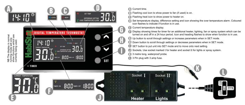
**SETTINGS**. Press the **SET** button and hold for 3 seconds. This puts the unit into SET mode. Use the **Λ V** buttons to change parameters (hold button down for rapid change) and then press **SET** to save and move onto the next setting. The order is shown below. Elements **highlighted** indicates flashing display.
