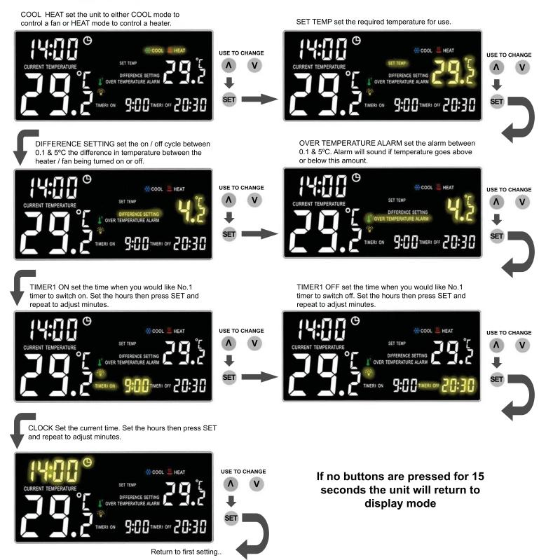
**Quick check of settings.** Settings can be quickly checked without going into the setting routine. Simply scroll up or down with the Λ V arrows. Functions will scroll through and will flash indicating current settings of those functions flashing. You cannot alter these settings in this manner and the normal display will resume if untouched for 5 seconds.
